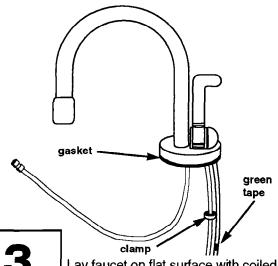
Lav faucet on flat surface with coiled tubing facing up. Using one hand to hold tubing just below faucet, carefully
